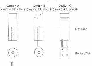
Note: Option C is the most widely used method of anchoring bollards.
