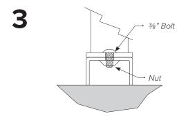
Put bolts through U BIKE RACK flange holes and beams so bolt head faces up. HAND tighten the nuts using new flange nuts.
