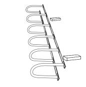
Once nuts are on, tip assembled rack over and use a 9/16" socket to tighten nuts. Before fully tightening nuts, make sure the racks are straight on beams. If using tamper resistant nuts, use access tool to tighten nuts. Do not overtighten the tamper resistant nuts. Tip rack upright.
