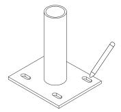
Place the rack in the desired location. Use a marker or pencil to outline the holes of the flange onto the base material.
