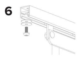
If no more Bike Files are going to be spliced together, insert a 3/8" Unistrut nut into the end of the channel and affix with 2 large washers and tamper-proof bolt. Finish by hammering in an End Cap.
