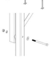
B) For double-sided units, fasten the Double-sided Uprights and Upright Braces to the Uprights with 3/8" x 3" bolts, 3/8" washers, 3/8" lock washers, and 3/8" nuts.
