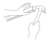
Insert a ½" Carriage Bolt into the last slot and fasten 3 Washers and a Tamperproof Nut. Finish by hammering in an End Cap.
