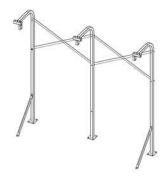
Fasten the Channel Supports to the uprights with ½" x 3" bolts, ½" washers, ½" lock washers, and ½" nuts.
