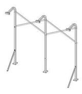
A) For single-sided units, attach Knee Braces to the first Upright and then every other Upright with  $3/8" \times 3"$  bolts, 3/8" washers, 3/8" lock washers, and 3/8" nuts. Anchor each Knee Brace by drilling a 3/8" hole and fastening with a wedge anchor.
