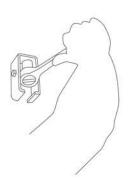
Mount Channel Trolley Supports in ceiling with appropriate anchors so that the centers of the brackets are 19" from each end of the 96" Slotted Track and 32" apart from each other.
