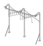
Insert the Track Rack or Bike File assembly into the Channel Supports and secure. See Track Rack or Bike File instructions for more detail. 4b
