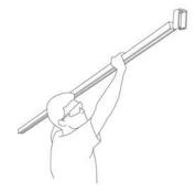
Slide 96" Slotted Track through the Channel Trolley Supports so that the centers of the brackets are 19" from the end of the Slotted Track
