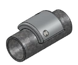
Drill 1/4" clearance holes on rail. Epoxy will create insular ring around fastener as it threads through tapped holes on bracket
