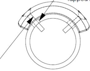
Tamper resistant screws are threaded through bracket and cross lock to rail. No tapping on rail is required.
